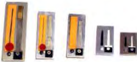
Figure 2: On the left, is shown a reed with an added mass, which permits to have lower frequencies keeping the same reed length.
